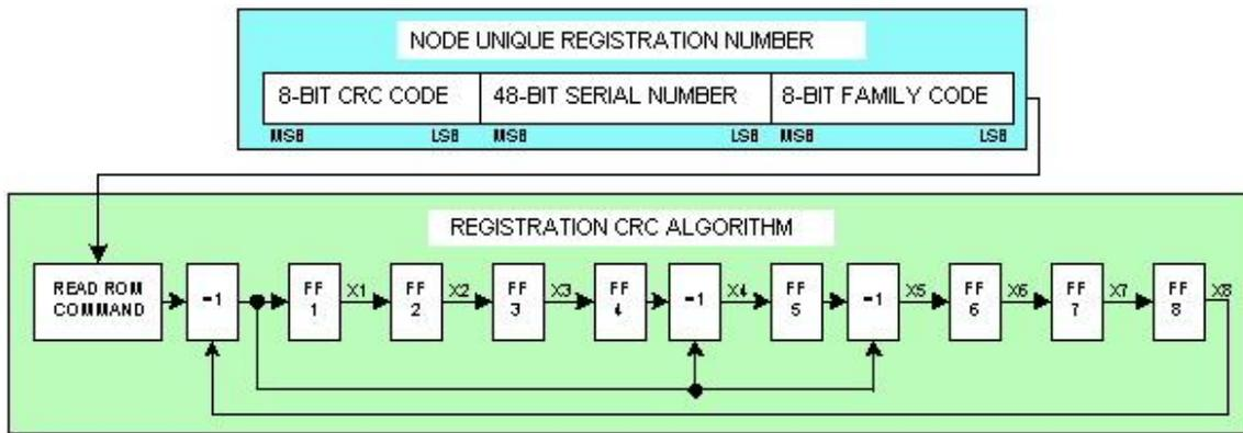
All IEEE 1451.4 transducers storing TEDS data in the transducer and transmitting that data on the mixed mode interface (MMI) must use a node(s) containing a URN(s).
