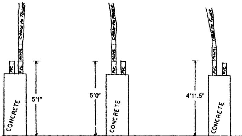
FRONT VIEW OF CONDUIT IN CONCRETE
