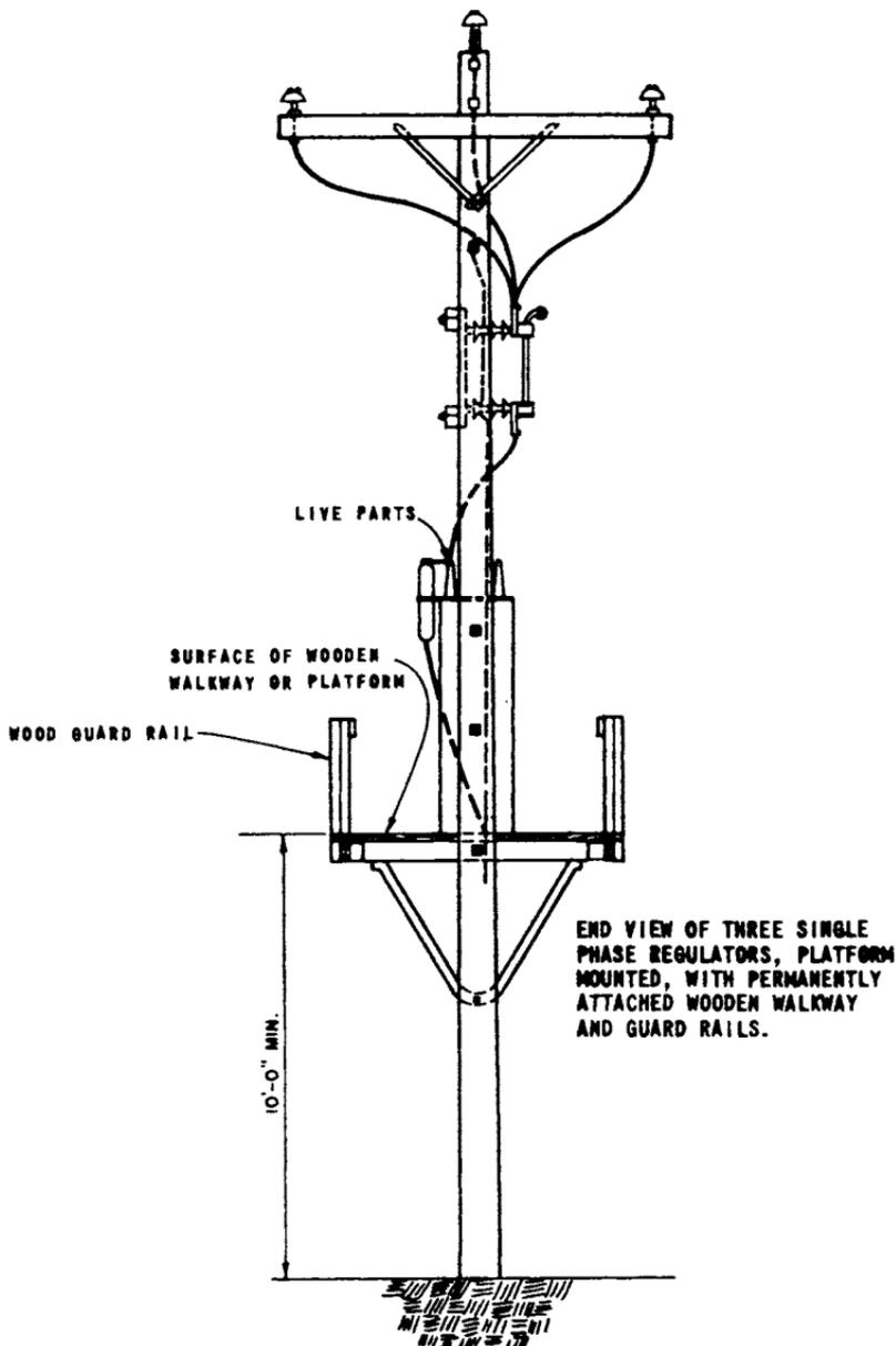
END VIEW OF THREE SINGLE PHASE REGULATORS, PLATFORM MOUNTED, WITH PERMANENTLY ATTACHED WOODEN WALKWAY AND GUARD RAILS.
