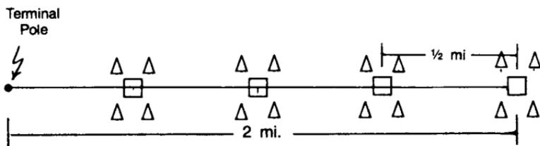
▲ ▲ Denotes 20' × 20' ground grid around each enclosure, calculated resistance of each grid 2 ohms or less in 2000 ohm-centimeter soil.
